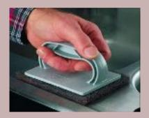
Abrasion or scuffing of the surface will in many instances enhance adhesion by increasing the surface area available for bonding. Scuffing must be followed by cleaning with IPA/water mixture.
