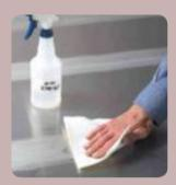
Most substrates are best prepared by wiping (in one direction) with a 50:50 mixture of isopropyl alcohol {IPA} and water or 3M hIPA Clean 300.
