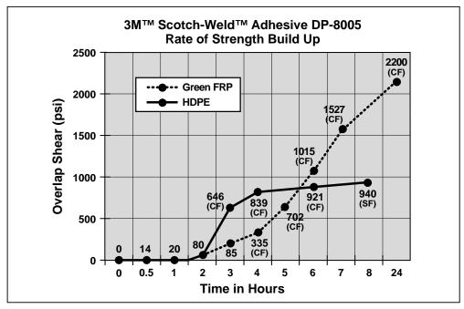
The above rate of strength build up was collected on 1" x 4" x 1/8" HDPE and Green FRP specimens overlapped .5", allowed to cure at 75°F (24°C) for 24 hours and then tested at a rate of .5"/minute in overlap shear mode, at 75°F (24°C). All values are reported in psi.
