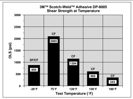
SF: Substrate Failure, CF = Cohesive Failure
