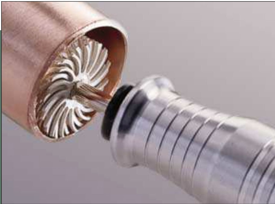
1" Radial Bristle Disc, grade 120, removing light mill scale and finishing inside of copper tube.
