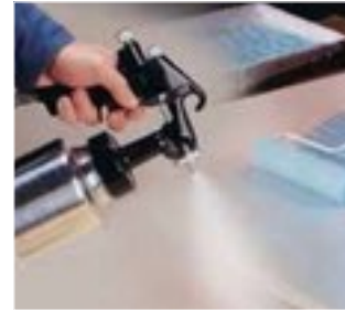
In cabinet assembly, 3M™ Fastbond™ Contact Adhesive 30NF is a proven formulation. Combining an open time of up to 4 hours with high immediate bond strength. Apply with roller, brush, or spray gun.
