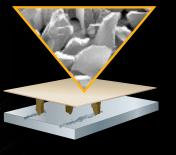
Conventional ceramic abrasive grain tends to "plough" through the metal, causing heat to build up in the workpiece and the abrasive — resulting in a slower cut and shorter disc life.
