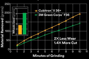
Data from internal testing on 1018 mild steel using 100mm flexible grinding wheels
